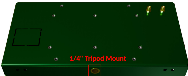
Figure 5. Underside of ESPARGOS One with the 1/4"-20 tripod mount highlighted.
