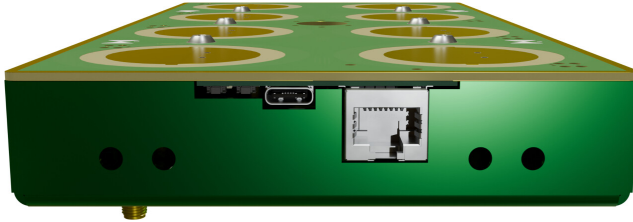
Figure 1. The side panel of ESPARGOS One with the RJ45 Ethernet and USB-C connectors.
